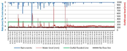
Figure 7: Dry flow water levels at 5-minute intervals at the STEM outfall for the week between the 28<sup>th</sup> of October and the 3<sup>rd</sup> of November. 2017.
